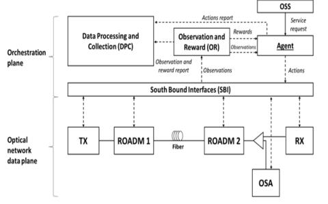
Work carried out with Politecnico di Milano optical group How many channels are allocated without disruptions?
