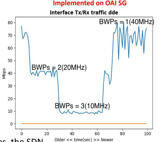
As the capacity requirement changes, the SDN controller reduces the bandwidth required (i.e., to save on bandwidth resources)
