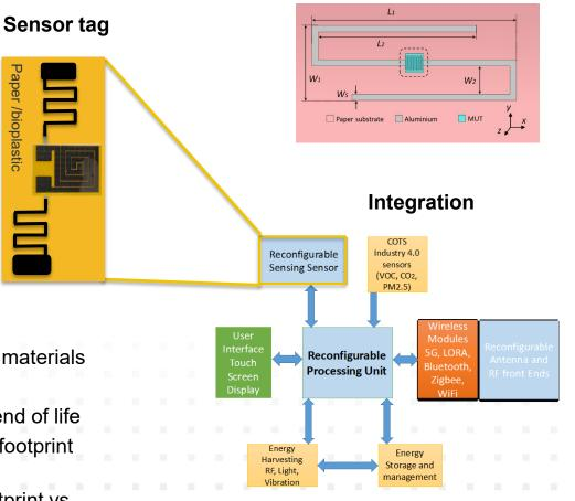
Flexible, reconfigurable energy autonomous sensing platforms for IoT networks
