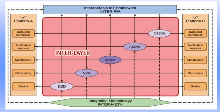
The INTER-LAYER tools will provide techniques and technology allowing interoperability and integration between the layers of heterogeneous IoT platforms
