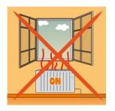
Window opening sensor prevents wasting energy while airing out
