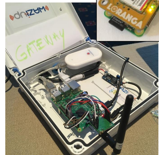
RPI 3 LoRa WiFi PoE 2G/3G dongle DHT22 in-case sensor
