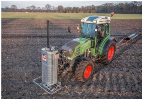
Electrical conductivity scanner detecting clay content and organic matter for conductivity zoning
